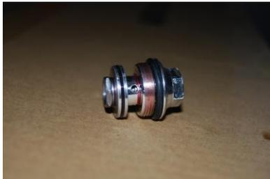
The compression damping unit consists the damping piston with shim stack and the adjuster seat with screw.
