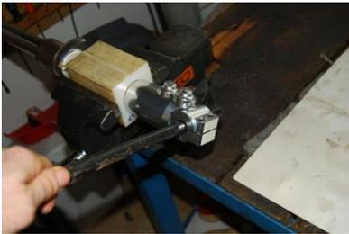
Back off the compression and the rebound damping adjusters. Loosen the lower foot out of the slider. It is secured not only by the lock screw but by thread bound as well, maybe needs heating to remove it.
