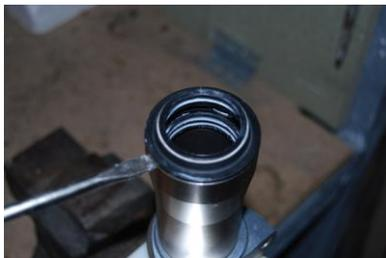
Dust seal, seal clip and oils seal can be removed from the slider for check and replace.
