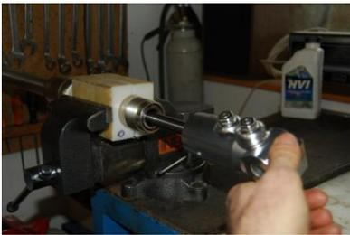
Now you can pull the lower foot with damping unit and the stanchion out of the slider.
