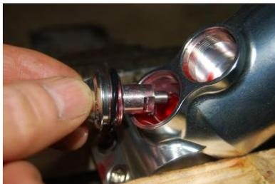
The rebound damping adjuster unit adjusts the control rod by it's conical screw.
