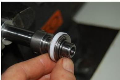
Remove the rebound valving and the damping piston
