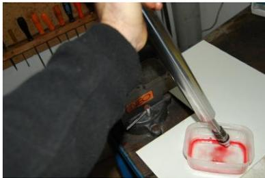
Turn over the stanchion, so the damper can slide out of it.
