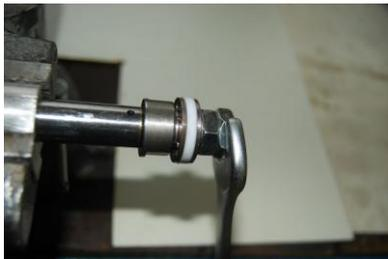
Clamp the damping rod in a vise again and loosen the nuts of the damping piston
