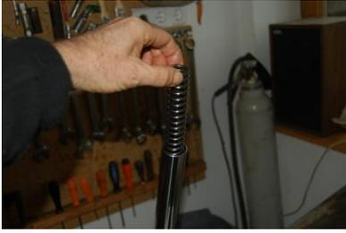
Remove the parts from the fork tube (washer, spacer, another washer and the fork spring) Pour out the fluid, each leg consists 250ml.
