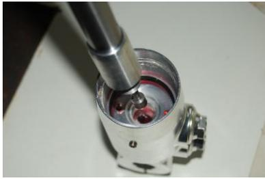
Take the stanchion-damping unit out of the vise, remove the bottom-out cone from the damping rod.
