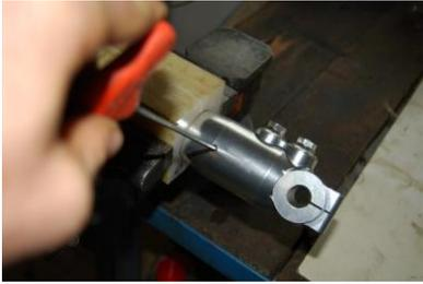
Align the lock screw of the lower foot
