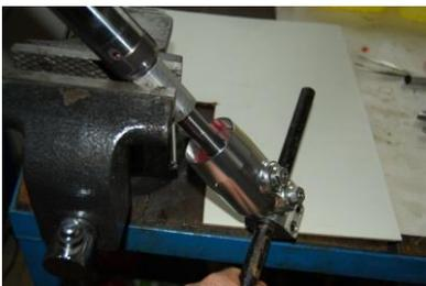
Clamp the damping rod in a vise with soft tool (in our case it's two half of an aluminium tube with 17mm inner diameter). Loosen the lower foot.
