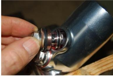
The compression damping unit can be also removed from the lower foot.
